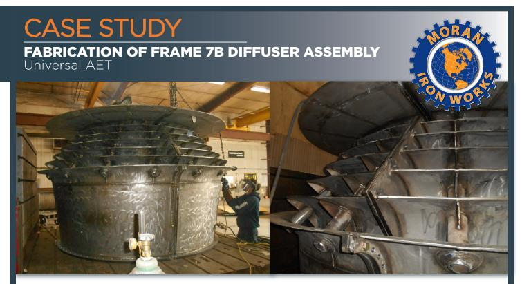
Moran Iron Works was awarded a contract to fabricate a replacement diffuser assembly for install at Universal AET's customer. This unit was fabricated using 304H, high carbon stainless steel, for durability in the extreme heat of a Frame 7B exhaust. Flanges to hold tight tolerances and shipped direct to the project site.
