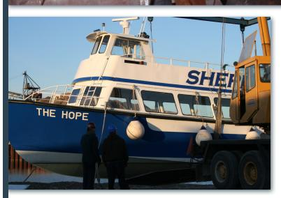
In 2009, Moran Iron Works performed a vessel overhaul and a mid body extension on Shepler's Mackinac Island Ferry's THE HOPE. In November 2009, the 69' aluminum monohull ferry was hauled out at Port Calcite and trucked to the main fabrication shop in Onaway. A 17' aft portion of the vessel was removed and discarded, and a new 35' section was fabricated in the shop and attached to the existing aluminum hull. The completed vessel is 87' long with an 18' beam.
