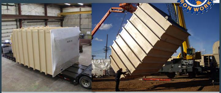
Moran Iron Works was awarded the contract to fabricate a complex silencer and plenum heat shields for a 40 plus year old Frame 5 unit. This silencer stack had three levels of
